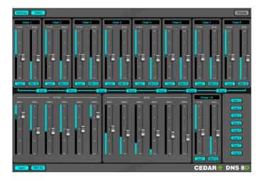
The DNS 8D incorporates its remote control software in the form of an internal web page, and you may connect to this using a suitable browser. To access it, connect the DNS 8D's control port to your Ethernet network. It will attempt to obtain an IP address from the network using DHCP and then register its serial number as its hostname. Once this is complete, enter the unit's address...
